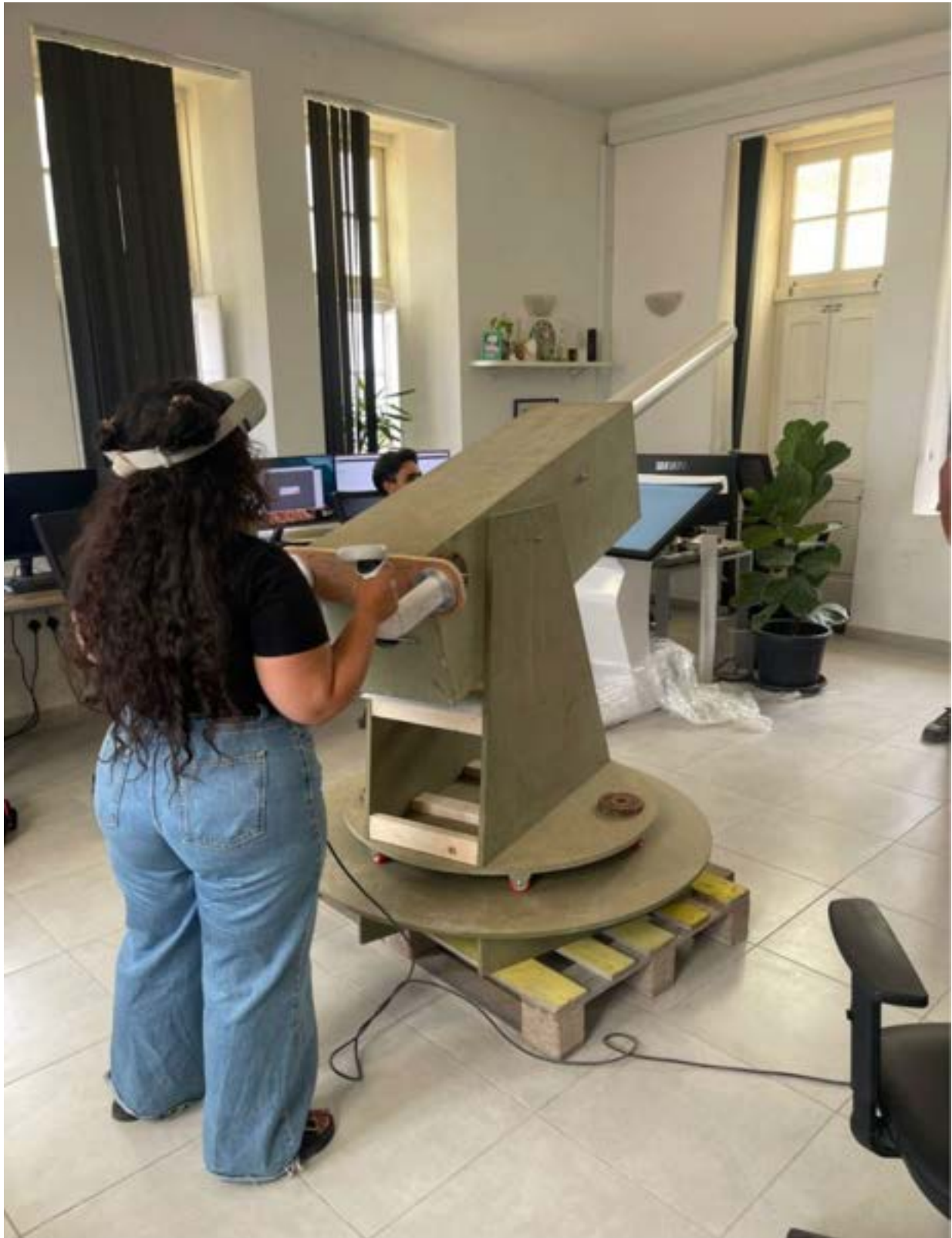
Figure 17. Prototype of the custom-made replica of the canon, used as an interface for the VR game.
