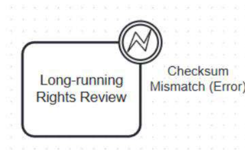
Fig. 9. BPMN boundary event symbols illustrating interrupting and non-interrupting variants attached to an activity.
