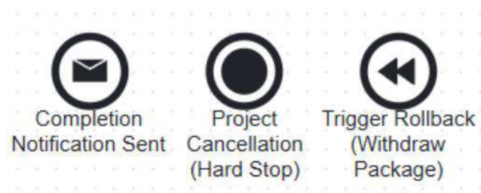
Fig. 8. Three BPMN end event symbols showing a message end event, a terminate end event, and a compensation end event.
