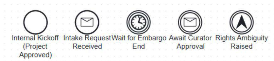
Fig. 6. Five BPMN event symbols showing a none start event, a message start event, a timer intermediate event, a message intermediate event, and an escalation intermediate event.
